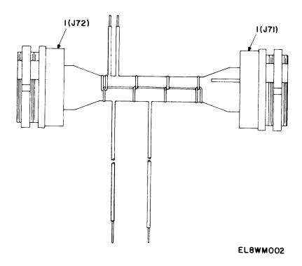
Figure 2. Wiring harness assembly SM-D-951293.
